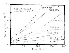
FIG. 5. The dependence of high temperature creep resistance of  $YL-Si_3N_4$  ceramics on different GB widths.
