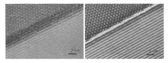
FIG. 6. HR-TEM picture of YL-Si<sub>3</sub>N<sub>4</sub> ceramics with different GB widths.
