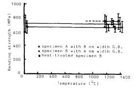
FIG. 4. The dependence of bending strength on temperature of  $YL-Si_3N_4$  ceramics with different GB widths.
